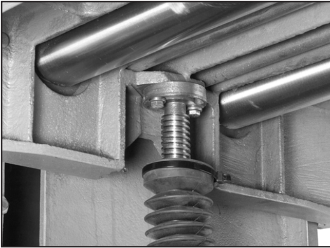
Figure 14. Column adjustment flange underneath table.
